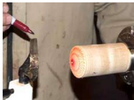
Chatter made easy: With one quick swipe of the chatter tool Rick adds texture to the end grain. Another brief stroke with a colored pen accents the pattern.
